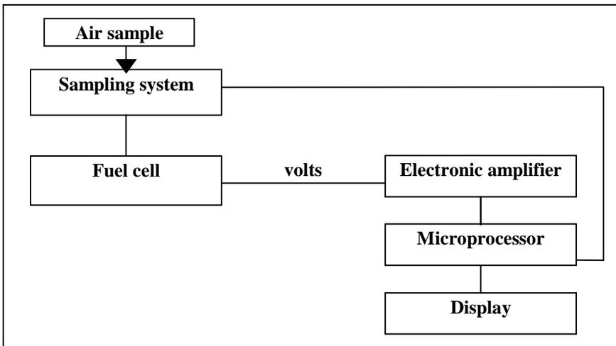
The instrument is simple to operate and may be used as often as required, provided that a suitable delay is allowed between successive tests.
