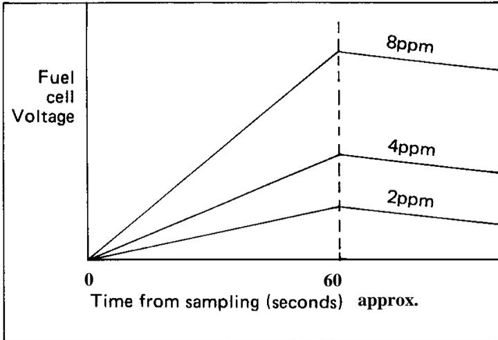
Since the fuel cell sensitivity will vary slightly with time, the calibration should be checked regularly. The fuel cell is guaranteed for 1 year.
