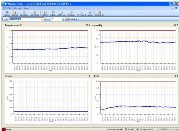
The collected data is presented on the controller PC in real-time. The graphical display enables the user to identify trends and patterns in the sampling; simple user interfaces enable easy use and operation of the software. The user can monitor and control each individual unit and sensor using the software. It is possible to create monitoring schedules using the software, which is ideal if monitoring only needs to take place for a set period of time (e.g. during rink opening hours only).
