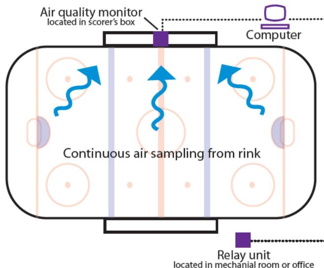
PPM Technology's wireless monitoring unit is installed in the ice rinks 'scorer's box'; the monitor continuously receives air samples from the rink, readings are transmitted in real-time to the rink office computer which stores the readings on easily read graphs.
